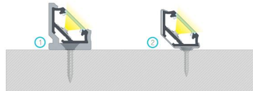
The result of assembly of corner profile C with a BASIC cover using plastic mounting clip CH
